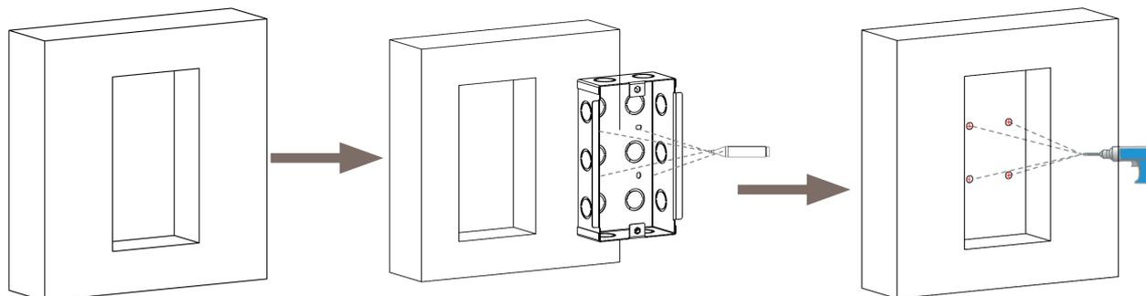
Cut a rectangular hole in the wall with dimensions 180x101x50. The hole should be slightly oversized to fit all the necessary cables.
