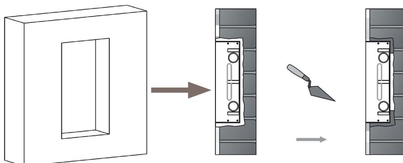
Cut a rectangular hole in the wall with dimensions 180x101x50. The hole should be slightly oversized to fit all necessary cables. Use cement or non-corrosive structural glue to fix the recessed box.
