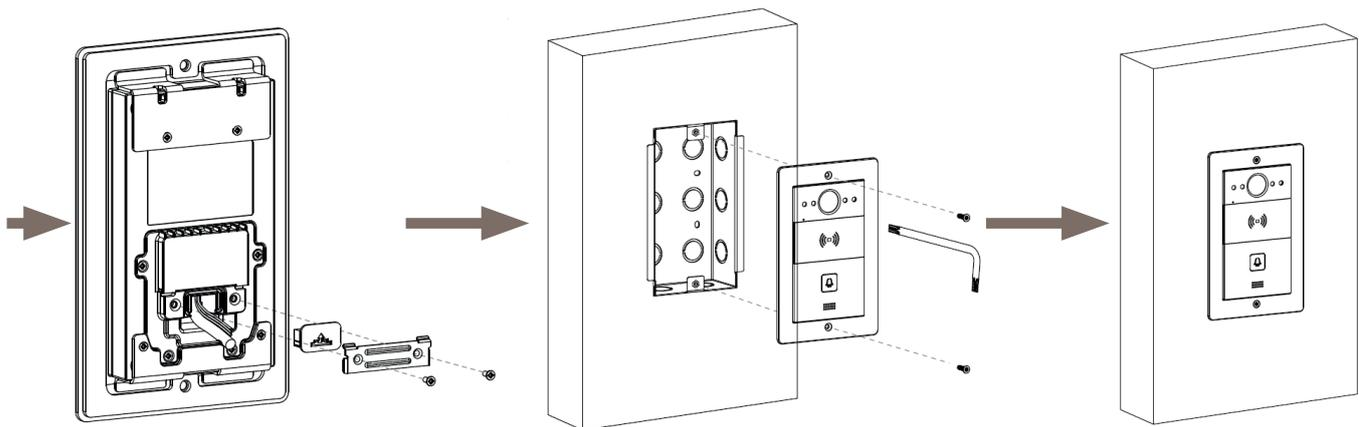
Choose a rubber plug of suitable size to push all cables into the cover. Attach the cable locking plate to the back cover using two M2.5x6 screws.
