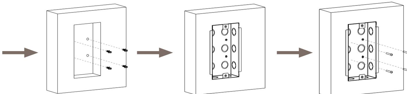
Insert four plugs into the holes.
