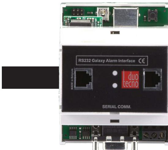
This interface can communicate with Honeywell's Galaxy G3 and GD (dimension) security system. With this interface, one can arm and disarm the alarm via Duotecno's touchscreens provided that one original code keyboard of the alarm is still present.
