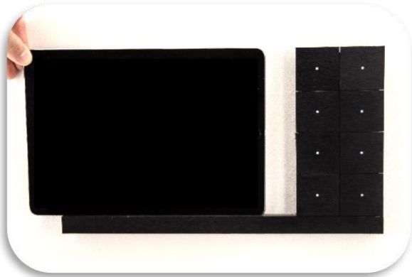
11. Mount the iPad by sliding it along the Eyeswitch bracket and clicking it in the lightning connector. Transparent sticker at the right back corner of the iPad for firmness
